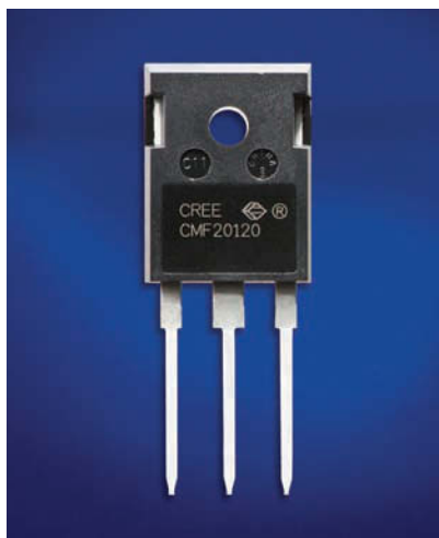
Figure 1 Cree's CMF2012SD series FETs compete with 900V silicon-based MOSFETs and 1200V IGBTs.
